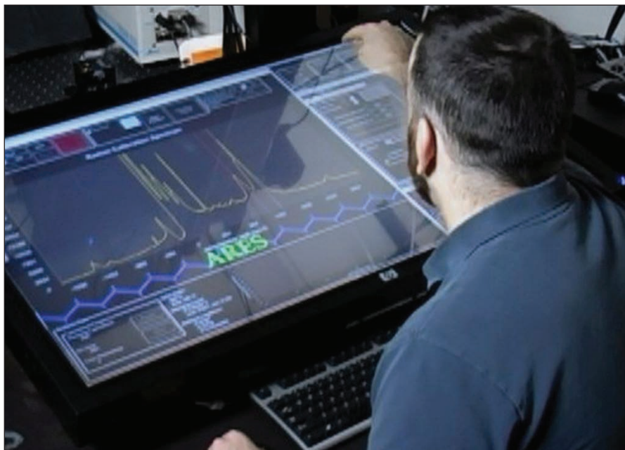
A materials researcher at Wright-Patterson AFB, Dayton, Ohio, examines experimental data on the ARES artificial intelligence planner. The ARES Autonomous Research System, developed by the Air Force Research Laboratory, uses AI to design, execute, and analyze experiments at a faster pace than traditional scientific research methods.
