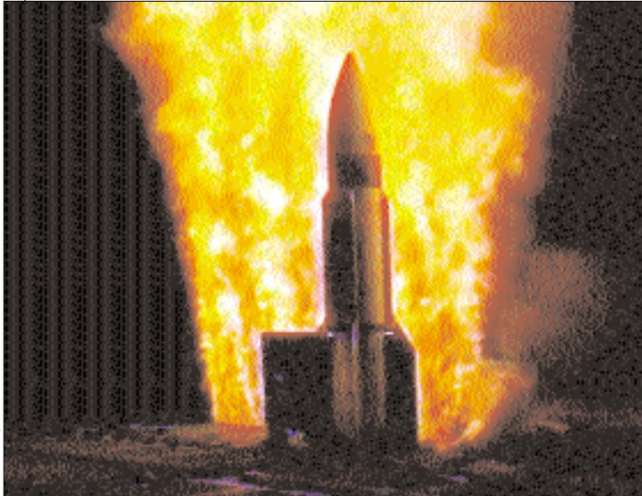
A Standard Missile (SM-3) leaving the vertical launch system of the cruiser USS Lake Erie during a January 2002 test of the new exo-atmospheric missile developed to counter theatre ballistic missile threats.
