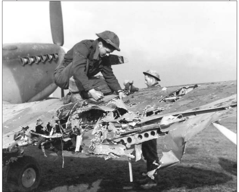
Repairing flak damage to an RCAF Spitfire, Holland, 1944.
