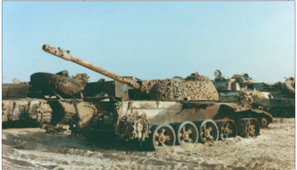
DU penetrator strikes on an Iraqi tank, presumably from the 30 mm GAU 8 mounted on A10 aircraft. Some larger penetrator strikes, possibly tank 120 mm APFSDS DU rounds, are also evident.
