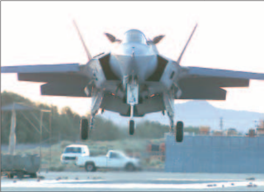
In 2001, a Joint Strike Fighter (JSF) X-35B demonstrator made a successful vertical take off test flight.
