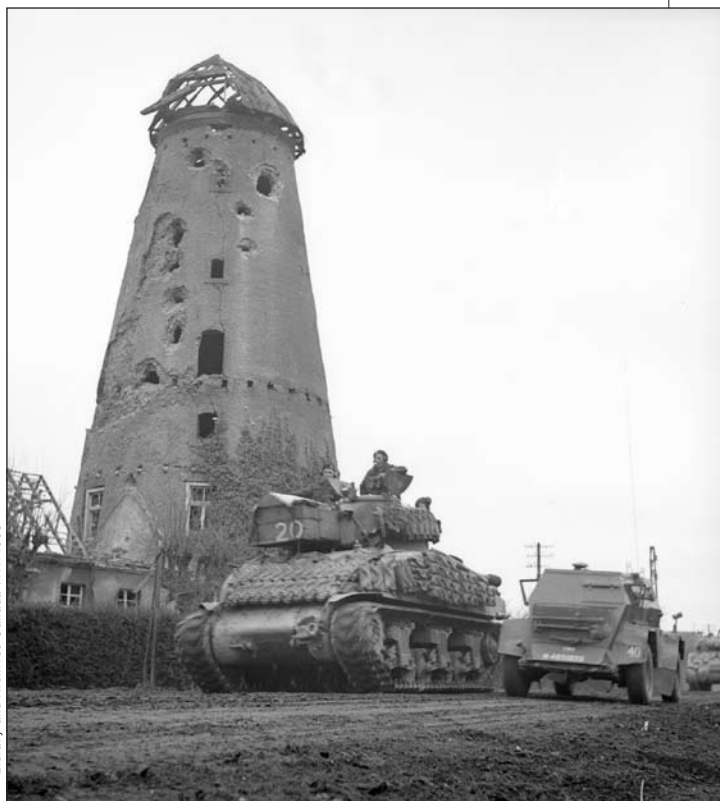
The Sherbrooke Fusiliers enter Xanten, Germany, 7 March 1945. The additional armour protection on the tank's hull is readily apparent.
